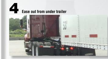
**EASE OUT FROM UNDER THE TRAILER.** Pull forward slowly until the fifth wheel clears the kingpin. Dump the air from the tractor suspension, and drive carefully away from under the trailer.
