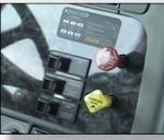
Open fifth wheel with release valve located on the dash or in a lock box mounted on the rear of the cab. To open, set the tractor parking brake and pull the release valve. Hold the valve open until the locking mechanism is locked in the
