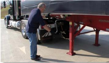
**LOWER THE LANDING LEGS.** Lock the trailer brakes, and back slowly into the trailer to ease pressure on the fifth wheel locking jaw. Engage the parking brake while the tractor is pushing against the kingpin. Then, chock the trailer wheels and lower the landing legs. Make sure that the trailer is positioned on a level surface that will support the weight of the trailer.
