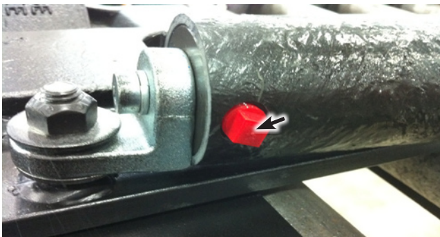
Figure 5: Plastic plug in air cylinder
