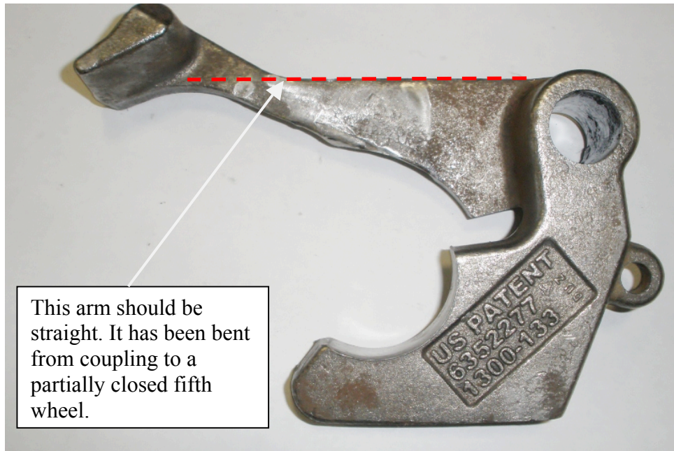
Damaged Rotating Jaw Caused By Improper Coupling Figure 5
