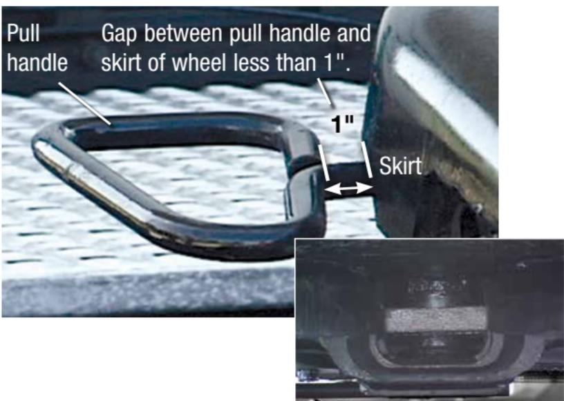
*Use a flashlight and go under the trailer and look into the back of the throat of the fifth wheel. The locking mechanism should be engaged across the entire throat of the fifth wheel and secured to the kingpin.*
