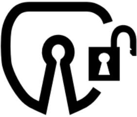
When the fifth wheel is ready to couple the “unlocked” indicator is illuminated in red (see FIGURE 10). If this is flashing, check to make sure fifth wheel is open prior to attempting couple.
