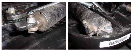
6000 & 7000 series fifth wheels including the Clean Connect Series). Be sure to follow the instructions included in the kit. Pay special attention to the mounting tab cylinder orientations and do not over torgue the fasteners.
