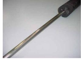
the air cylinder forward a small amount. This will allow the cylinder shaft to be extended by hand. Do not use the pull valve in the cab of the tractor to extend the cylinder. Clean the shaft of the cylinder removing any dirt or grime that has built up. WD40 can be used to aid in cleaning the cylinder shaft.
